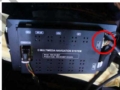
Connect a supplied LVDS cable to "1CH LVDS-IN" port of the supplied monitor
