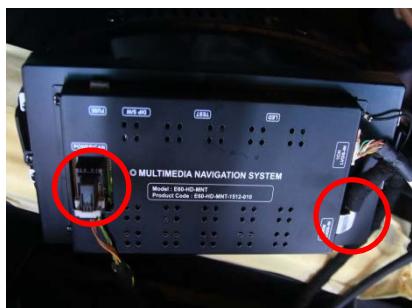
Connect OEM cables to the marked place as shown above
